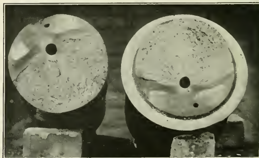
Fractured Crank Pin Discovered by Means of the Detector.
